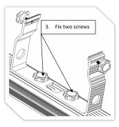
Step 2: Slide bracket into slot of driver box to right position s hown as following:
