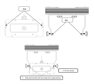
Step 3: Fix hanging kits onto driver box and hang LED bar fixture at right height.
