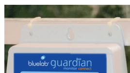
Cable ties fixed through small mounting holes around a support or bar.
